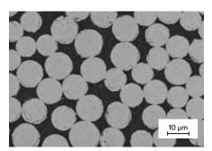
Fig. 2: SEM image (magnification 2kx) of a cross-section of RelyX<sup>\*</sup> Fiber Post 3D Glass Fiber Post. Glass fibers are depicted as white spots surrounded by a composite resin matrix. Source: 3M Oral Care internal data.
