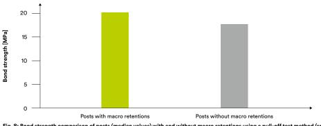
Fig. 8: Bond strength comparison of posts (median values) with and without macro retentions using a pull-off test method (speed: 1mm/min). Bonding surface treated with Scotchbond<sup>™</sup> Universal Adhesive. Filtek<sup>™</sup> Bulk Fill Posterior Restorative light-cured from front side for 20 s, samples were stored (1h 36 °C/>95% rel. humidity; 23 h water 36 °C) prior to testing. Source: Schwarz et al.<sup>7</sup>
